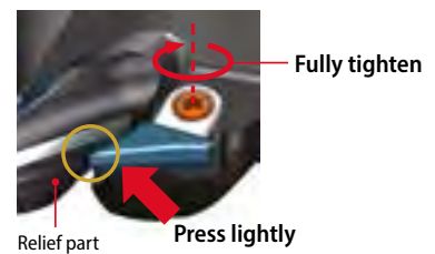
Fig.5 Fully tighten
