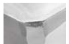
Competitor F After machining 11 m
