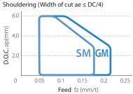
Cutting conditions: Vc = 150 m/min, ae = DC/4 mm, Workpiece: S50C
