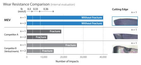
$Cutting\ conditions: Vc = 120\ m/min, ap \times ae = 2 \times 10\ mm, fz = 0.3 - 0.36\ mm/t, \\ \emptyset 20\ (1\ insert), Dry\ Workpiece: SCM440\ \textcircled{+}\ (37\sim39HS)$
