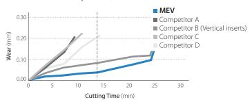
$Cutting\ conditions: Vc = 180\ m/min,\ ap \times ae = 3 \times 10\ mm,\ fz = 0.1\ mm/t,\ \varnothing 20,\ Dry\ \ Workpiece: SKD11\ (30\sim35HS)$
