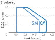
Cutting conditions : Vc = 150 m/min, ae = DC/2 mm, Workpiece : S50C
