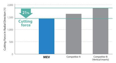
$Cutting\ conditions: Vc = 200\ m/min, ap \times ae = 3 \times 18\ mm, fz = 0.10\ mm/t, \\ \varnothing 20\ (3\ inserts), Dry\ Workpiece: SCM440\ (House, SCM440\ Moreover, SCM44$
