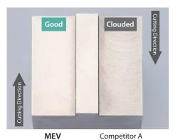
Cutting conditions : Vc = 180 m/min, ap  $\times$  ae=3  $\times$  40mm, fz = 0.1 mm/t, ø50 (5 inserts), Dry Workpiece : S50C
