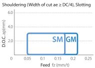
Cutting conditions: Vc = 150 m/min, ae = DC mm, Workpiece: S50C
