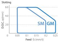
Cutting conditions: Vc = 150 m/min, ae = DC mm, Workpiece: S50C
