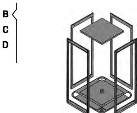
The Practibox swivel shelf consists of a 360° swivel base that houses 4 Practibox drawer unit holder frames, available in 3 different heights. Capacious, robust, practical – characteristics that make it usable in both large and small spaces.
