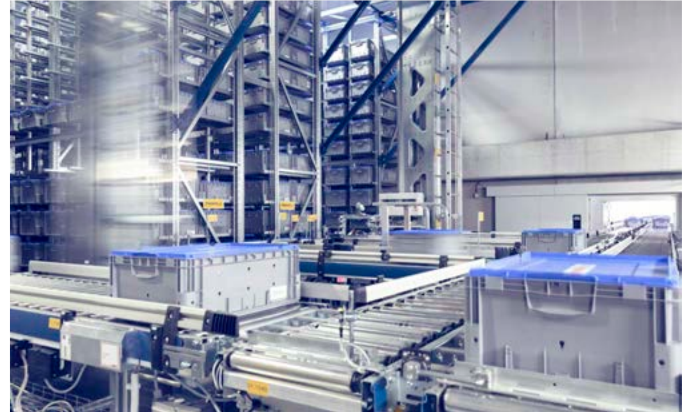
The 3 stacker cranes handle 10.000 iMiLOG Space boxes sized 600x400 mm 220 mm in height and 18.000 boxes 280 mm in height, with a 50 kg capacity. Boxes are complete with barcode + RFID and colour logo with IML In-Mould-Labeling process.
