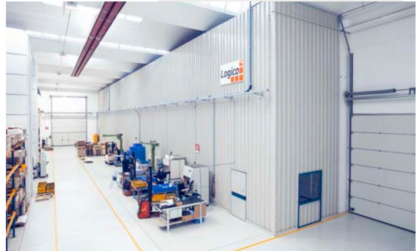
Integration of automatic warehouse within the manufacturing area.
