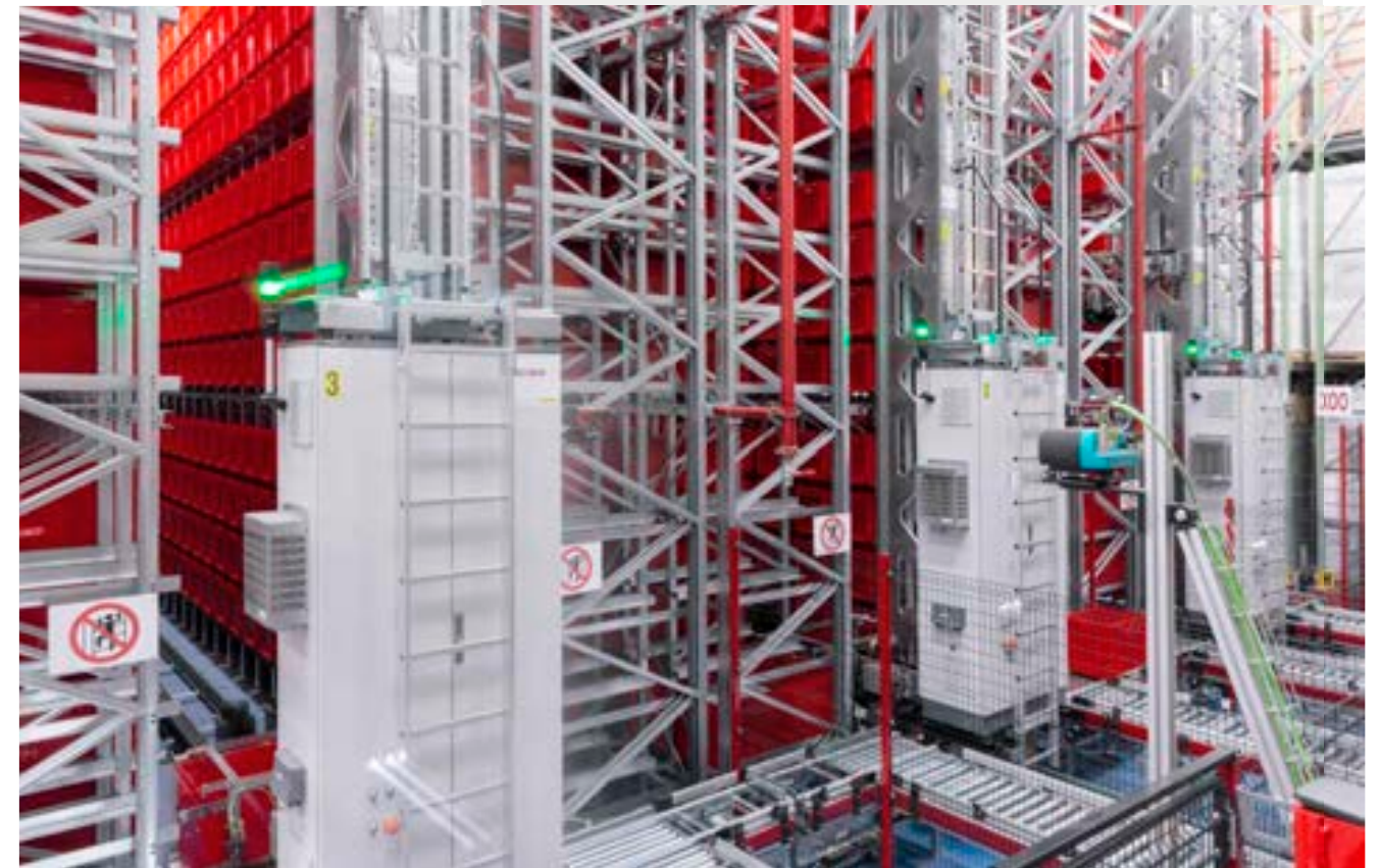
The 3 stacker cranes handle 5.500 iMiLOG Space boxes sized 600x400x420h mm, with a 50 kg capacity.
