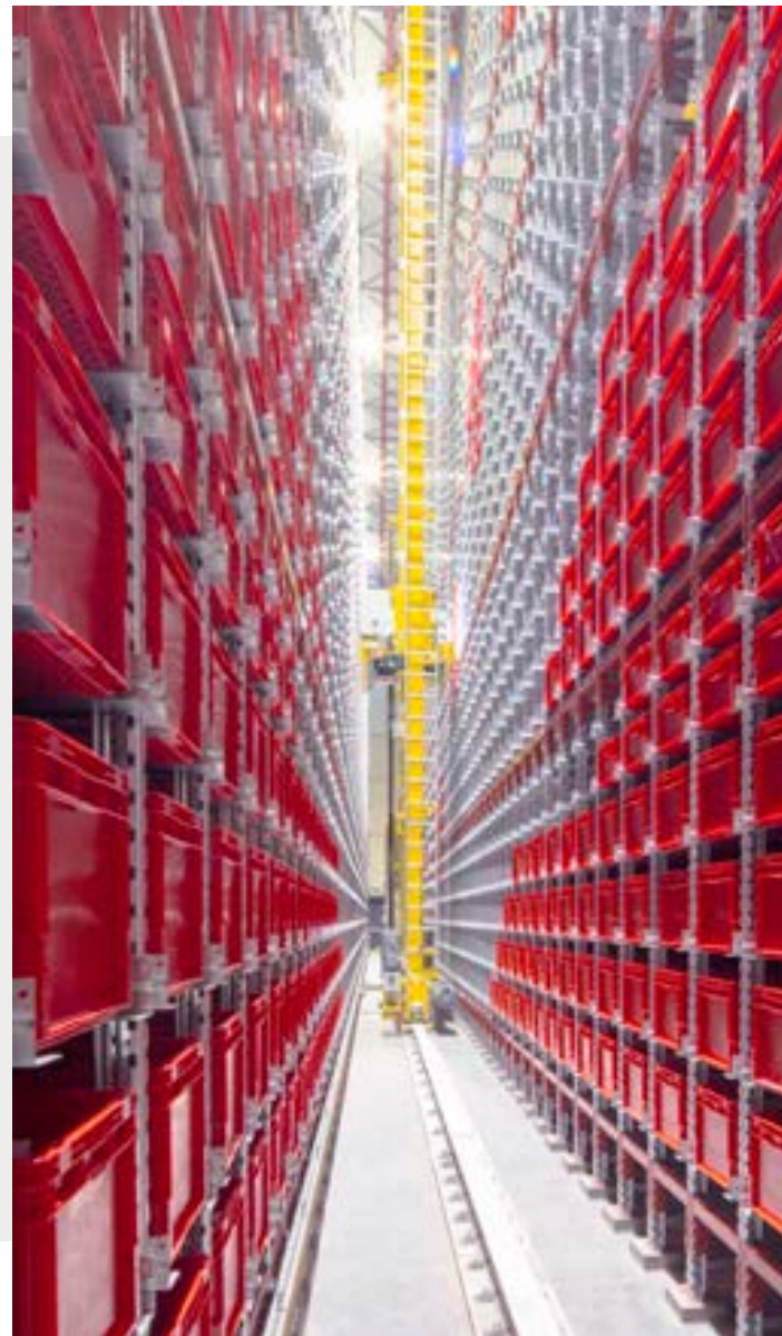
Automatic self-supporting warehouse with 3 stacker cranes handling 28.000 iMiLOG 600x400 mm Space boxes, 220 and 320 mm in height, with a 50 kg capacity and internal partitions. Another 2.500 iMiLOG Nest 600x400x320h mm boxes are used for distribution to BI ESSE subsidiaries.
