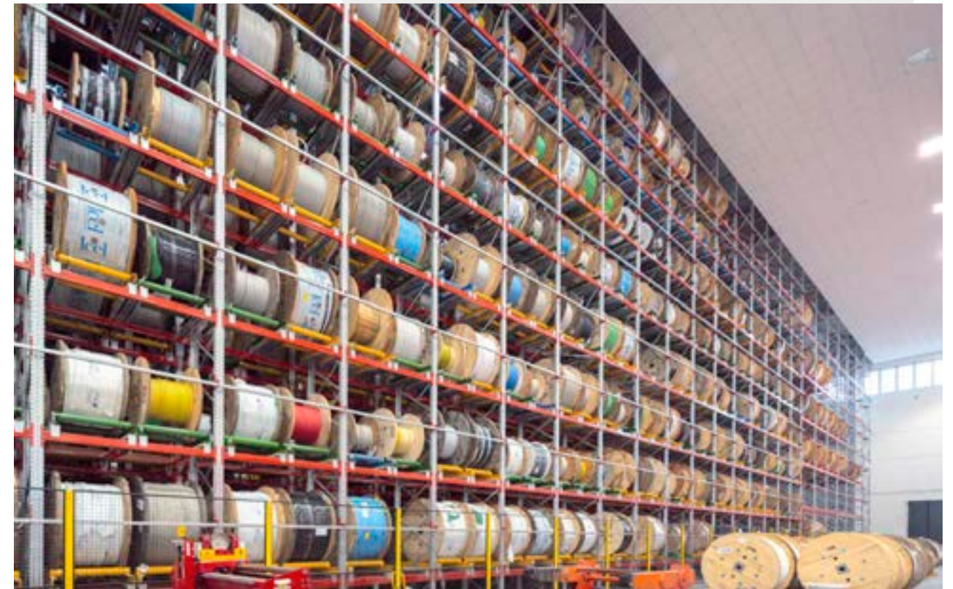
Automatic warehouse for cable reels with dual depth stacker crane.
