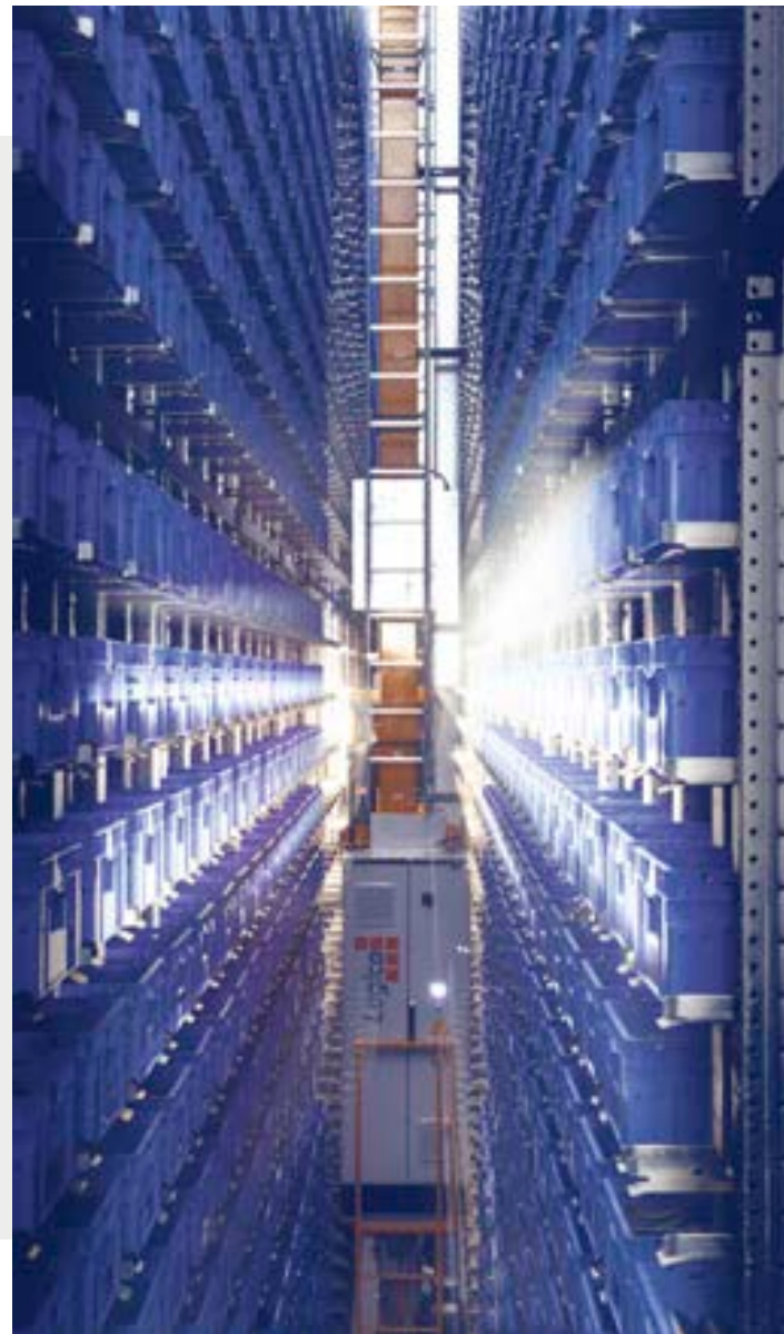
Automatic warehouse with stacker crane for 5.682 iMiLOG Odette boxes sized 600x400x220h mm and 2.448 boxes sized 600x400x320h mm, with a 100 kg capacity.
