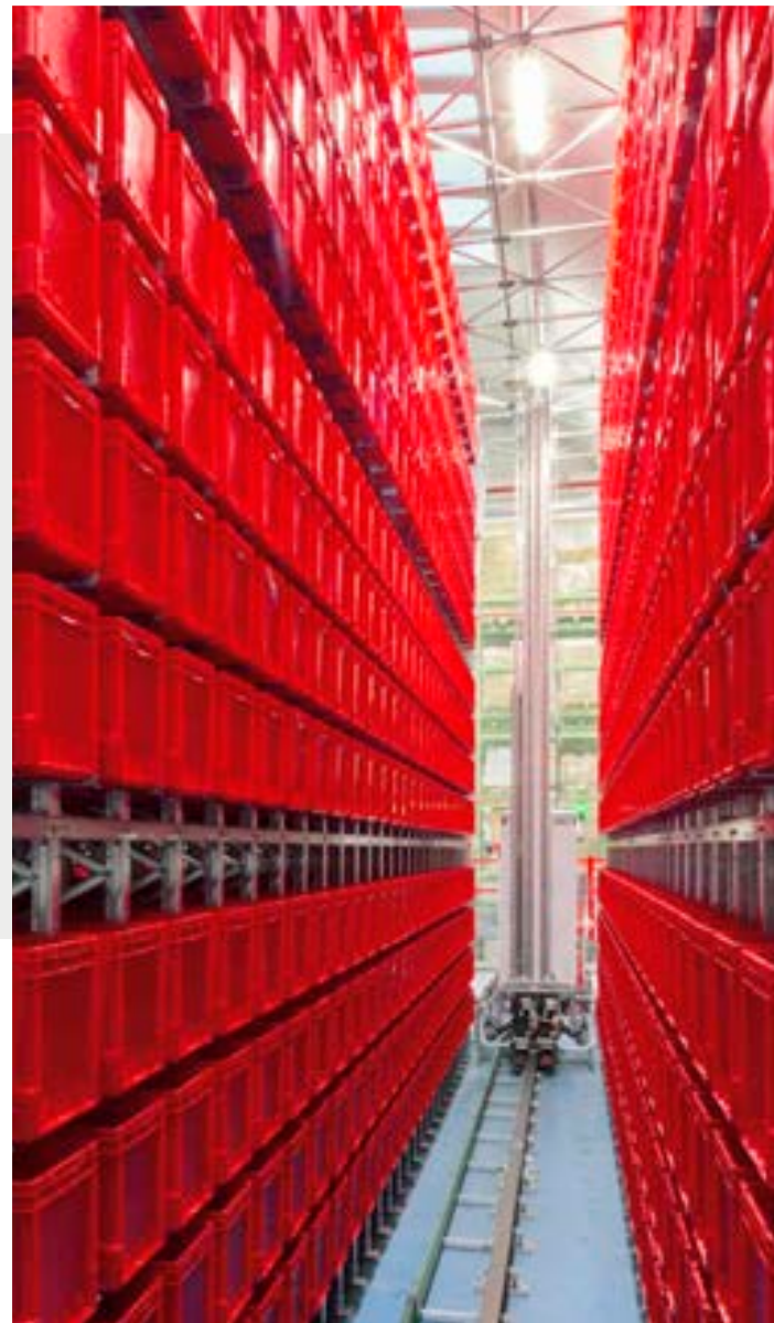
Automatic warehouse for boxes with 3 stacker cranes.
