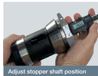
Lock stopper shaft and install
