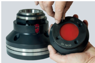
Remove bar seal from housing
