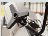
Saw band break monitoring The saw band tension is fitted with a saw band tension and saw band monitoring device
