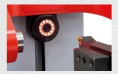
**EZturn for IC1, IC2 and IC3** To achieve optimal tooling results and longer tool lives, rotary tools must be set to their maximum height. EZset offers an optional additional monochrome camera for this purpose — to set the rotary center of tool cutting blades. The camera's cross hairs can be rotated and moved.
