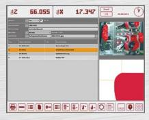
Data output in a format appropriate for the tooling machine controller (DOP), including format generator to generate post-processors / output formats (over 100 output formats are included in the EZset DOP library)
