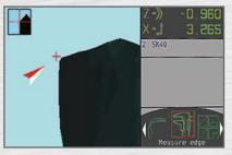
Compass needle — easily position the camera to measure target values on the tool
