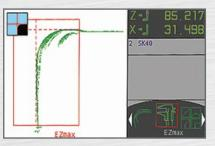
EZmax software function to determine and measure the maximum contour of the tool
