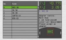
EZset zero point monitoring for 100% precise measurements after every adapter exchange
