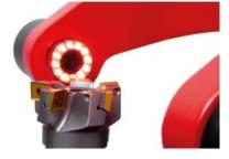
**Long-lasting LED Cold Light Source** for cutting edge inspection is standard on EZset tool presetting devices.
