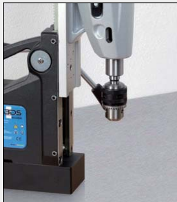
2. Place drill chuck in MT arbor.
