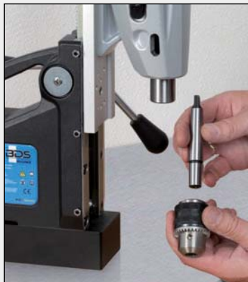
1. Connect taper drift to drill chuck.
