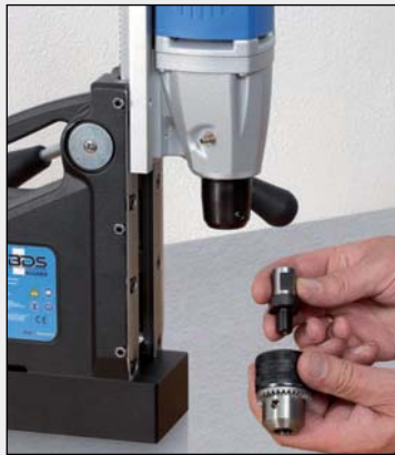
1. Connect adapter to drill chuck.
