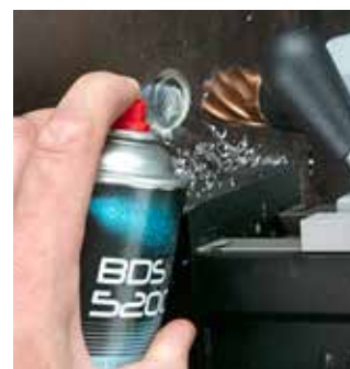
Step 2: During drilling, spray the high-performance lubrication spray onto the tip of the drill and into the cut hole.
