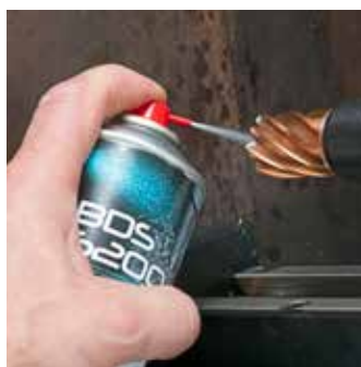
Step 1: Prior to drilling, spray the high-performance lubrication spray directly into the drill.
