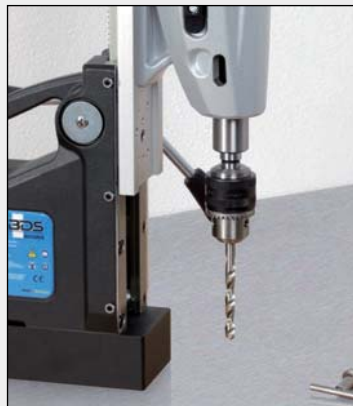
3. Ready for use with twist drill.
